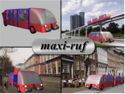
The solution to the problems was found to be the dualmode concept, i.e. the vehicles are able to drive in two different modes: on roads or on a special, exclusive monorail.
