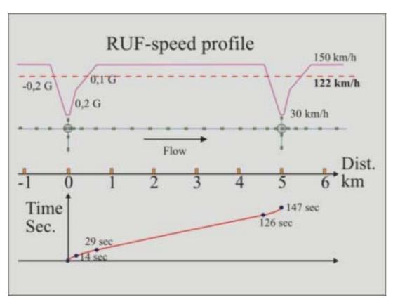
RUF has a fixed rhythm in the network of monorails. Access and egress is at a speed of 30 km/h. The top speed is 150 km/h and at every junction the speed is lowered to 30 km/h so that RUF can switch between monorails or leave the system.
