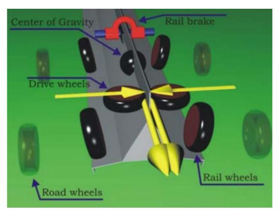
The drive system allows adjustment of the pressure against the monorail. This means that friction can be increased when it is needed i.e. when the vehicle accelerates or climbs a hill.
