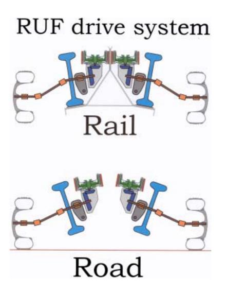
The drivesystem is built around 2 electric wheel motors which can be pressed against the top of the triangular monorail.
