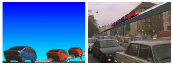
The egress ramp is placed as far away from freeway ramps as possible in order to avoid road congestion problems. If possible it will end close to a parking facility which can function as a buffer in case of problems. If an egress ramp get blocked, the ruf will be redirected to the next exit and will have to drive back from there (3 miles max.).
