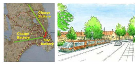
A RUF "tram" solution is much more attractive. It consists of a "train" of maxi-rufs and/or midi-rufs coupled together to form a "tram". No rails are needed because it runs on rubber wheels. No overhead wires are needed because it runs on battery power. This is possible because the vehicles makes use of the rail network in order to recharge the batteries in between the tram trips.
